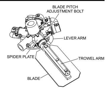
Figure 31. Blade Pitch Adjustment Bolt
